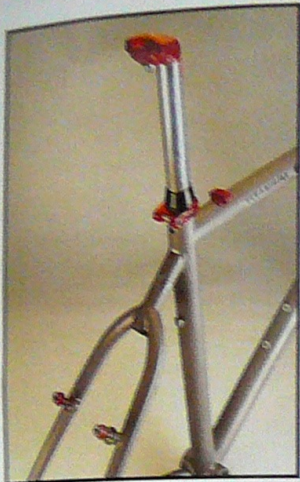
Wishbone seat stays, dedicated Seat Clamp and Tolerance Related Seat Post!
