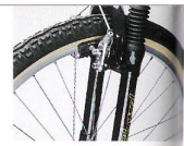
TopCap Elastomer Fork - 55mm of plush travel.
