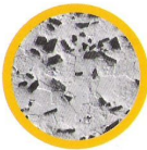
Microscopic view of M2 Metal Matrix Composite.
