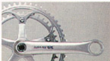
Crank arm is offset against spider arm for increased durability.
