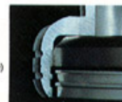
Sectional View of Rotating Head Part (Labyrinth Seal)
