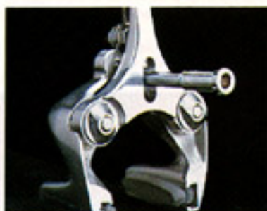
Sliding adjustable brake
