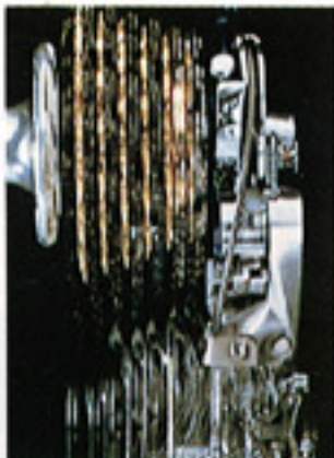
The built-in Positive Indexing Mechanism of the rear derailleur provides continuous top to low gear changes.
