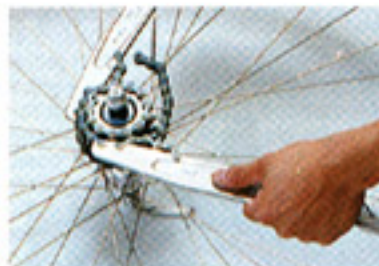
When removing sprockets, as seen in photograph, use the double wrap sprocket turning chain for easier operation.
