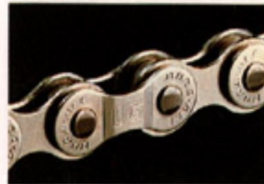
The UG Chain. Outerplates are widened to the level of chainpin heads.
