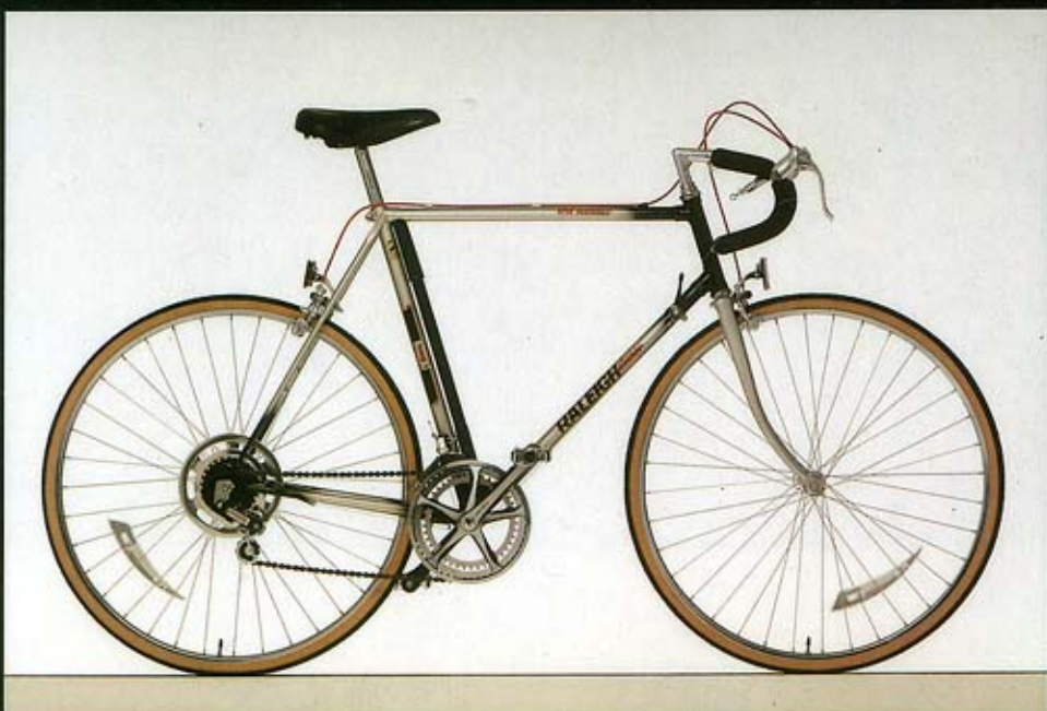
Brazed-on top tube cable guides
