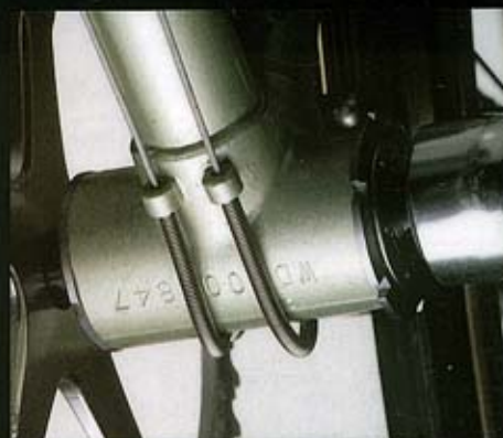
Under bottom bracket, cable guides and frame number
