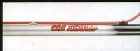
Brazed-on top tube cable guides
