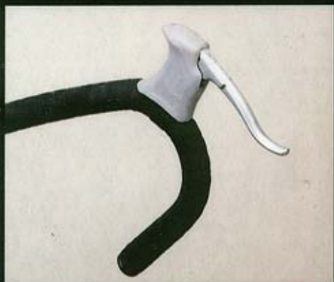
Shimano Adamas hooded levers with concealed cables
