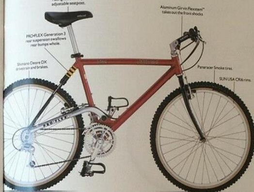
PRO-FLEX 962 FEATURES RIGID CROMOLY FORK & FLEXSTEM XST
