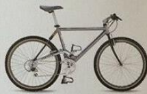
PRO-FLEX 962 FEATURES RIGID CROMOLY FORK & FLEXSTEM XST
