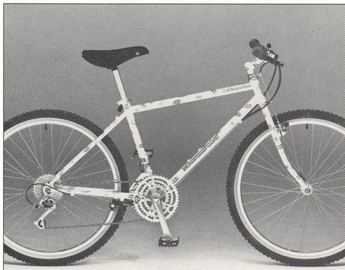
The Escape Goat uses the same geometry as the Deluxe, with cost efficient TIG welded construction, as a standard feature. Kisses optional.
