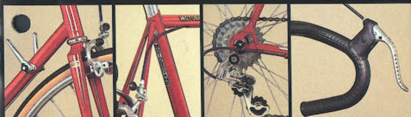
1 - ITALIAN DESIGN DROP SHOULDER FORK CROWN AND WEINMANN 501 SIDE PULL BRAKE. - 2 - RACING TYPE SEAT POST BINDER SYSTEM AND TAPERED REAR STAYS. INTERNAL BRAKE CABLE. - 3 - NEW HURET PILOT DERAILLEUR AND VERTICAL DROPOUT TIPS. - 4 - MOTOBECANE UNIQUE HANDLEBAR SLEEVES WITH HOODED DRILLED LEVERS.
