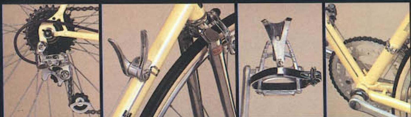
1 - SUN TOUR ARX DERAILLEUR AND VERTICAL REAR DROPOUT. - 2 - SUN TOUR SHIFTERS AND ITALIAN RACING TYPE FORK. - 3 - MAILLARD PLATFORM PEDAL AND PROFILE NERVAR CRANKSET. - 4 - BRAZED-ON CABLE GUIDES AND BOTTLE BOSSES.
