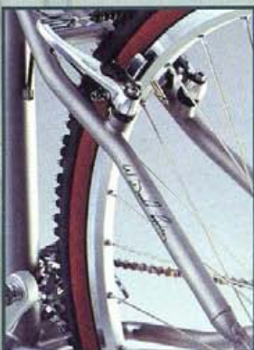
Unique S-bend seatstays add extra stiffness, tire clearance and braking power.
