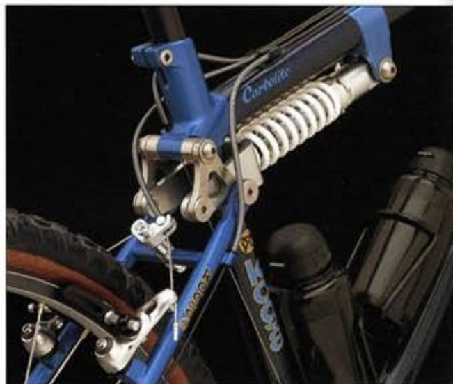
Koga-Miyata's instelbare suspensie systeem (RDG-S).
