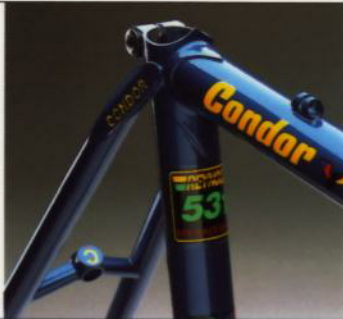
a A very rigid construction using solid top eyes.
