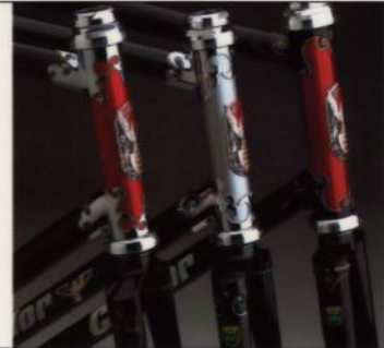
c An array of hand-crafted head lugs and fork crowns. The models are shown in the following order left to right: Superbe, No 1 and Elite.
