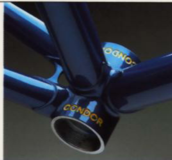
b A cast bottom bracket helps to perfect the strength of the frame.
