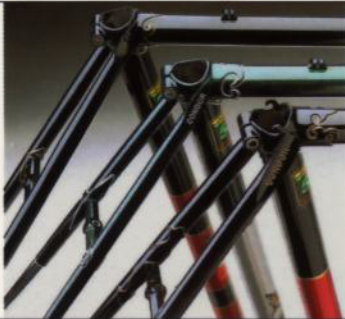
a Elegant designs of seat lug and brake bridges. The models are shown in the following order front to back: Superbe, No 1 and Elite.
