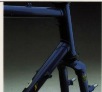
c Quality lugs and strong fork crowns incorporating cantilever bosses.
