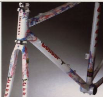
b Aero cast fork crown and all welded frame construction.
