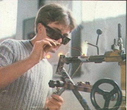
Brazing of fittings Inspection of brazed parts by liquid penetrant
